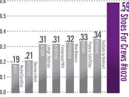
On a scale where 0.0 is the absence of friction and 1.0 is very high friction (e.g., dry carpet), SFC rated .59 – more than doubling the .29 average of the competitors above. See full April 2012 Independent Lab Test results at shoesforcrews.com/technology
