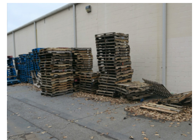
Do not store wooden pallets near your building
